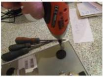
Remove the 5 screws on the front and back of the module that secure the bottom plate. This includes the two large slot-headed screws on the back of the
