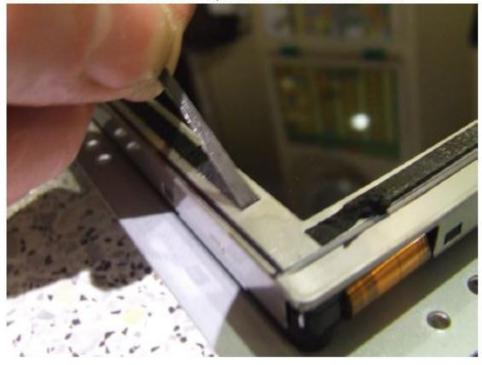
After completely removing the remains of the double-sided foam, replace the foam with new double-sided sticky tape or foam (sorry, not very clear on the photo below). Take care not to cover any of the TFT display glass with tape:
