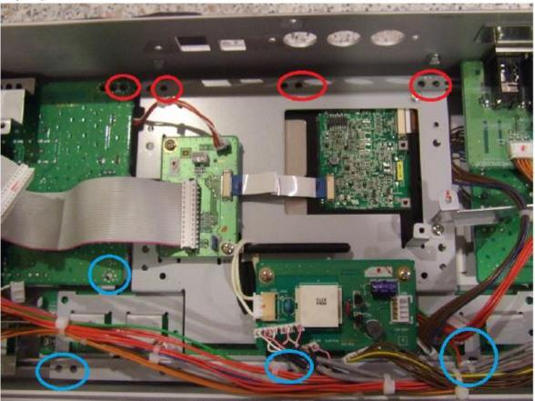
Remove the two end screws that hold the metal work at the LCD module end of the power supply board (to the left of the picture above). It should be possible to lift the end of the power supply nearest the LCD module slightly.
