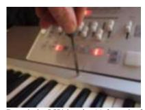
Detach the LH1 bracket(s) from the frame at the rear. Lift the module clear of the keybed.
