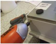
Carefully lift the bottom plate away from the unit. It is still attached by the cable connecting to the keybed connector. Disconnect this cable:
