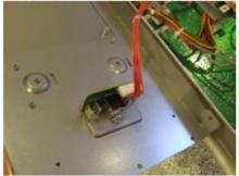
Now you can remove the bottom plate from the module, and keep to one side.
