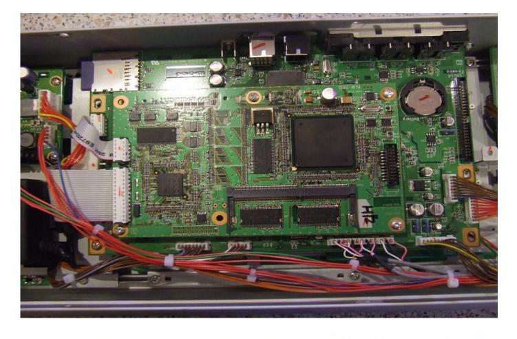
To start removing the main board, carefully disconnect the 7 connectors highlighted in yellow below. The large LCD flex connector on the left of the picture is the hardest to remove (Note: when I removed the main board, I started by removing the screws, then removed the connectors, however I think removing the connectors first is probably safer!). When disconnecting the connectors, take care not to bend the boards at all:
