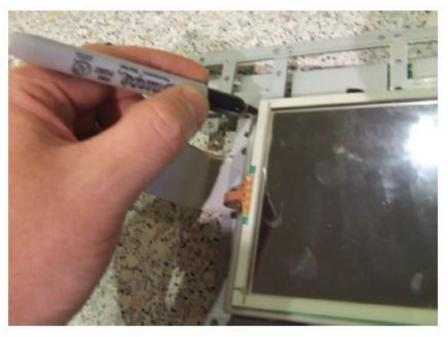
Pay close attention to what side the existing screen is showing. The new screen will need to be installed the same way, green color side closest to LCD, otherwise the connector will be wrong side up and no connection will be made to the LCD.
