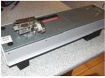
With a <u>Philips</u> screwdriver, remove the 3 screws on each side of the bottom plate at each end of the module. These screws are longer than the others in the module, so keep these separately:
