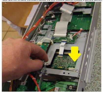
Remove the 6 screws that hold the LCD module to the top of the module, plus the two screws at the end of the switch / power supply board to the left (in the photo):
