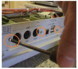
You should now be able to lift out and remove the main board (note that I took this photo prior to removing the connectors):
